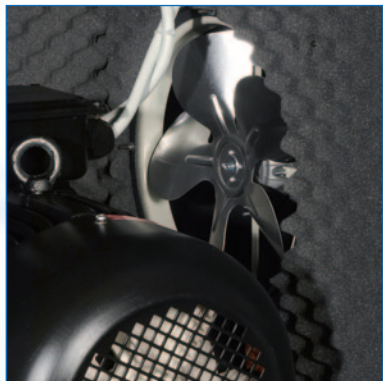
Cooling with extra electric fan (on 7,5 and 10hp)
