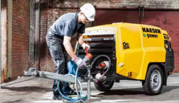
The new M 27E, M 31E and M 50E portable compressors truly come into their own wherever an electrical power connection is available. Their near-silent electric drive makes them the perfect choice for use in low emission and noise protection zones. The effects of noise from compressed air applications in tunnels or inside buildings are tamed by the compressors' emissions-free drive.
