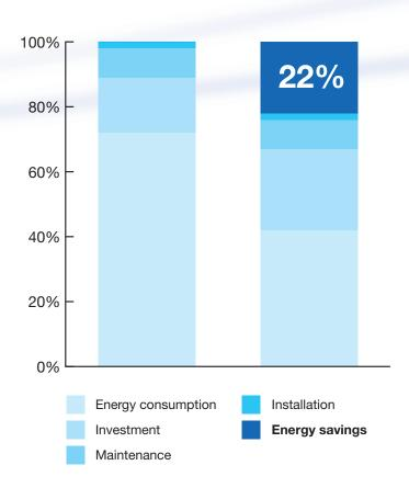
Air consumption within the network is not constant over time. A variable speed compressor lowers the speed of the motor according to the compressed air consumption. In this way, you can achieve major electricity savings.
