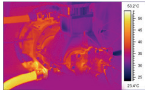
Limited temperature increase of only 25° C inside compressor element
